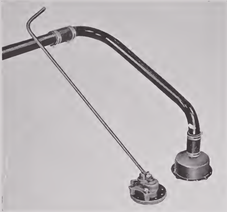
FIGURE 21. Drain valve with extension handle (left), shown with bilge suction cup (right).
